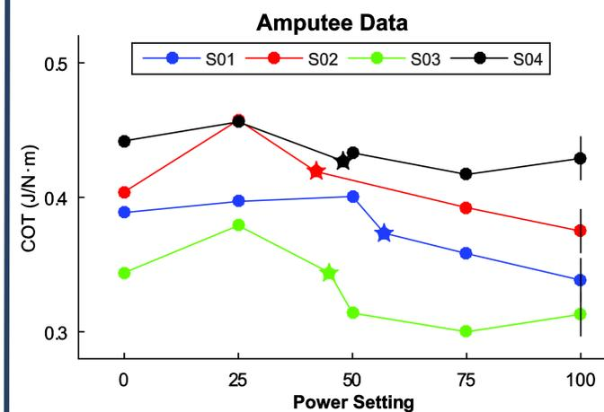
Figure 4. COT for 3 minutes of steady state walking with a solid line representing ± MDC (0.017 J/N.m) on 100% power and a star representing PC power
