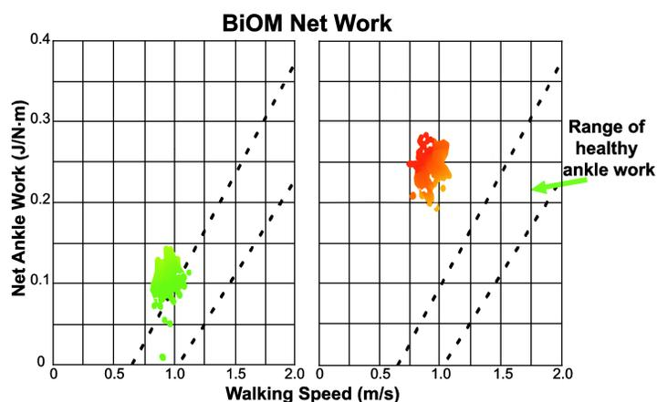
Figure 1. Example of tuning graph of BiOM with different power settings
